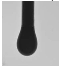
FIGURE 8 Goutte de lait+encre tensioactive pendante
